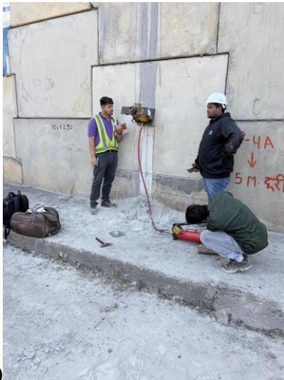
Figure 5 Photographs taken during trial nail installation and pullout testing
