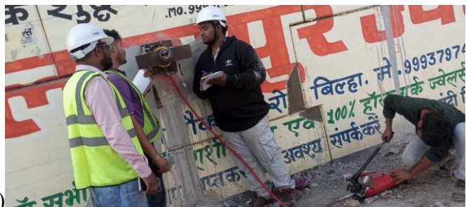
Figure 5 Photographs taken during trial nail installation and pullout testing
